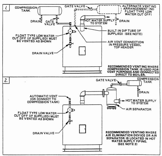
On hot water heating applications it is essential to eliminate as much air as possible from the system. Shown above are two methods of accomplishing this:
